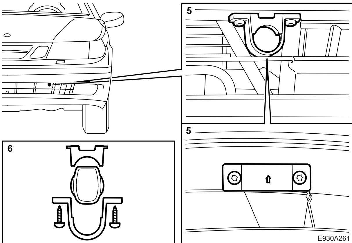
5 -M05: Mark out the location for the holder for the supply connector plug. The arrow on the holder should point forwards. Make holes with a bradawl.
