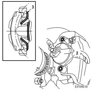
5 Apply 30 06 442 White high-pressure grease paste to the hub.
