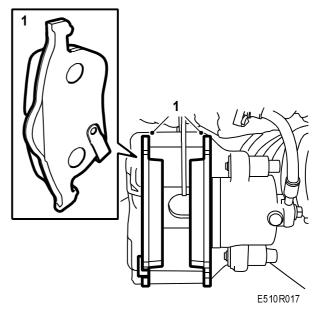
2 Fit the brake caliper, clean the guide pins and tighten them using a torque wrench.
