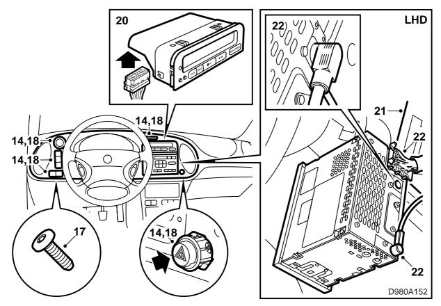
13 Lift the new instrument plate into position.
