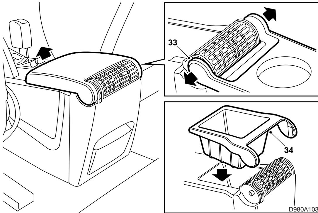
27 Remove the storage tray in the centre console between the seats.
